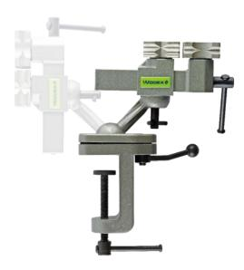
Adjustable aluminium alloy vices for mould makers and model makers, fitted with spherical joint that can be locked in any position by means of a quick clamping lever at the base. This solution means that the operator can maintain a correct and safe working position. Suitable for finishing or polishing work on delicate, small and medium-sized mechanical parts. Fitted with swivel grips for clamping irregular pieces.
