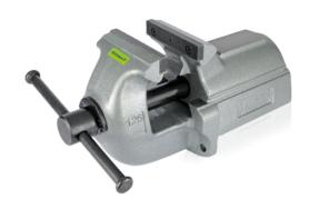
Bench vices **PREMIUM QUALITY** made of high quality cast iron with replaceable induction hardened and ground jaws. Designed to provide long service even for heavy duty use. Dovetail guides mean that the movement of the upper and lower guides is play-free, the upper part can be precision-adjusted using the screw. Fixing 3-point, 2 front and one upper. Grey painted with hammered finish.
