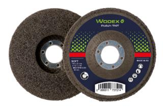
Non-woven disc impregnated with abrasive grit on a fibreglass backing plate. Close mesh allows minor imperfections left by flap discs to be removed for a perfect mirror finish.
