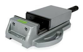
Vices for column drills **PREMIUM QUALITY** made of high quality cast iron with replaceable induction hardened and ground steel jaws. The prismatic jaws allow flat and round pieces to be clamped, while the sliding guides for the mobile jaw act as a support base for the precise closure of the pieces. Fixing more than 2 points. Grey painted with hammered finish.
