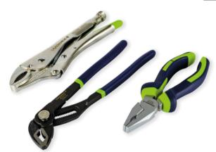
Set of PREMIUM QUALITY pliers containing a pair of universal combination pliers in chrome molybdenum steel, a pair of adjustable pliers with fine adjustment in chrome-vanadium steel and a pair of self-locking pliers in chrome-vanadium steel with concave jaws for clamping flat and round materials.
