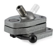
Fixing system with swivel and adjustable spherical joint. The aluminium alloy base can be fixed to a workbench, while the pin has an internal and external thread to receive special clamping devices made by the user. The ball joint can be locked into the required position using the quick clamping lever. Base with fixing of more than 4 points.
