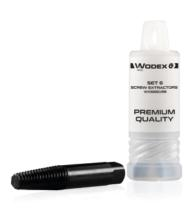
Set of conical extractors in chrome-vanadium steel for the removal of broken screws and studs that cannot be gripped. The WX5880 extractors can only be used on right-hand threaded screws and require a pre-hole for inserting the tool.
