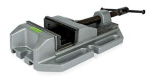
High quality cast iron vices for column drills **PREMIUM QUALITY** with replaceable induction hardened and ground steel jaws. The prismatic jaws are reversible, one side has a knurled surface and the other is smooth with a prismatic profile for clamping flat and round pieces. The sliding guides of the mobile jaw serve as a support base for the precise closure of the pieces. Fixing more than 4 points.
