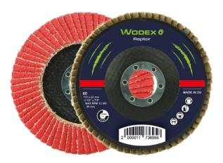
Flap discs with fibreglass backing and polycotton abrasive cloth with the latest generation self-lubricating ceramic abrasive grit. Monolamellar feature with conical backing pad. Outstanding ceramic abrasive removal capacity with cooling additives to ensure a cool cut. For heavy duty use, especially on high alloy and stainless steels.
