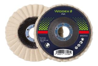
Felt flap discs with fibreglass backing plate. Specifically designed for use with abrasive paste in surface mirror polishing. Use on angle grinders at 2500 rpm (16 m/s).
