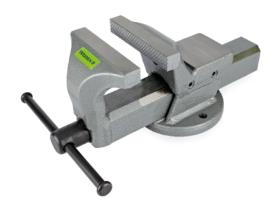
Bench vices **PREMIUM QUALITY** in high quality forged steel, front opening, non-removable induction hardened and ground jaws. All sliding parts are hardened and adjustable. Fixing more than 2 points. Grey painted with hammered finish.
