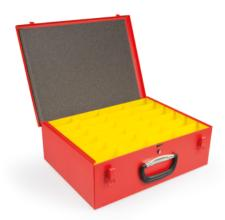
Small parts cases in epoxy coated sheet steel with practical carrying handle, lid with internal sponge to prevent small parts from falling out of the special containers, double lever closure and additional central spring closure against accidental opening. The cases are fitted with removable plastic containers for the optimal division of the contents.
