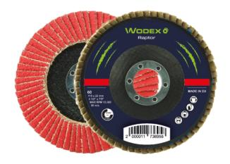
Flap discs with fibreglass backing and polycotton abrasive cloth with the latest generation self-lubricating ceramic abrasive grit. Monolamellar feature with flat backing pad. Outstanding ceramic abrasive removal capacity with cooling additives to ensure a cool cut. For heavy duty use, especially on high alloy and stainless steels.
