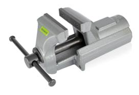
Bench vices **PREMIUM QUALITY** in high quality forged steel, rear opening, replaceable induction hardened and ground jaws. Play-free movement of the upper and lower parts thanks to the precision dovetail guides. Fixing 3-point, 2 front and one upper.
