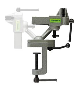
Adjustable aluminium alloy vices for mould makers and model makers, fitted with spherical joint that can be locked in any position by means of a quick clamping lever at the base. This solution means that the operator can maintain a correct and safe working position. Suitable for finishing or polishing work on delicate, small and medium-sized mechanical parts.
