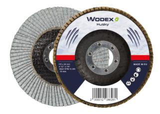
Flap discs with fibre backing and zirconium stearate cloth. The stearate allows cold working and lower disc clogging. Ideal for low pressure machining of aluminium cast iron, brass, copper and all clogging materials.
