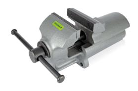
Bench vices **PREMIUM QUALITY** made of high quality cast iron with replaceable induction hardened and ground jaws. Play-free movement of the upper and lower parts thanks to the precision dovetail guides. Fixing 3-point, 2 front and one upper. Grey painted with hammered finish.
