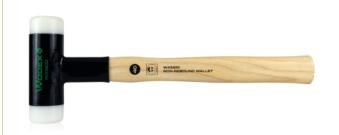
Mallets with replaceable polyurethane heads, head partially filled with metal pellets to absorb rebound, painted steel body and ash wood handle.
