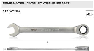
Combination ratchet wrenches with 144T fine teeth in chrome-vanadium steel, hardness 42-48 HRC, high torque transmission, 2.5° return angle, high resistance chrome-satin steel finish. Compliant with RoHS and REACH directives.
