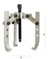
Mechanical extractors **PREMIUM QUALITY**. In traction it engages automatically with the parts to be extracted. Jaws with extension holes. Grooved ends for possible attachment to a screw. This series of extractors is designed to be used even with only 2 jaws. Chrome-satin finish.
