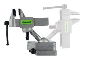
Adjustable aluminium alloy vices for mould makers and model makers, fitted with spherical joint that can be locked in any position by means of a quick clamping lever at the base. This solution means that the operator can maintain a correct and safe working position. Suitable for finishing or polishing work on delicate, small and medium-sized mechanical parts.
