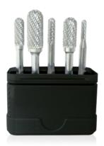
Selection of 5 rotary burrs, including G6050, 6mm shank cut 6. Cylindrical shape with spherical head. Suitable for machining all materials of various strengths, ideal for machining surfaces, profiles and for the pre-milling of build-up welds.
