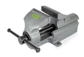
Bench vices **PREMIUM QUALITY** in high quality forged steel, rear opening, replaceable induction hardened and ground steel jaws. Play-free movement of the upper and lower parts thanks to the precision dovetail guides. Fixing more than 3 points. Grey painted with hammered finish.
