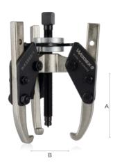
Mechanical pullers **PREMIUM QUALITY** with 3 self-centring jaws, external model with forged jaws and extension holes. Fitted with simultaneous jaw closing device. This series of extractors is designed to be used even with only 2 jaws (apart from sizes N.5 and N.6).
